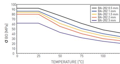
σ<sub>BO</sub> diagrams represent σ<sub>BO</sub> values for different gasket material thicknesses. These values indicate the maximum in-service compressive pressures which can be applied on the gasket area involved without destructing or damaging the gasket material.
